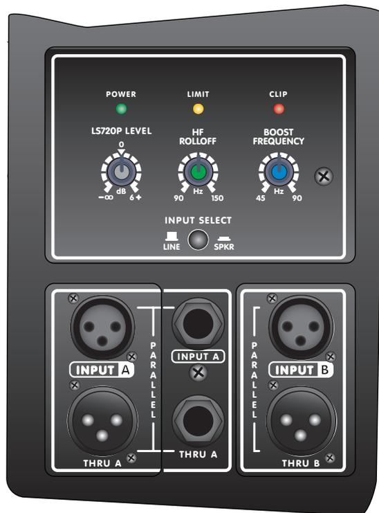
*At high power levels when the limiter is operating, increasing the subwoofer level control will not increase the output. Do not increase the setting while operating at high levels.*
