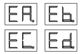
Different elements can be selected for editing by pressing the appropriate [ELEMENT SELECT] key — [A], [B], [C] or [D]. If a 2-element voice is being edited, only elements A and B can be selected.
