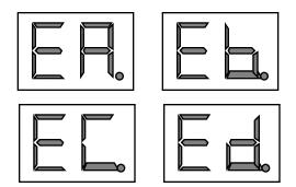
Different elements can be selected for editing by pressing the appropriate [ELEMENT SELECT] key — [A], [B], [C] or [D]. If a 2-element voice is being edited, only elements A and B can be selected.
