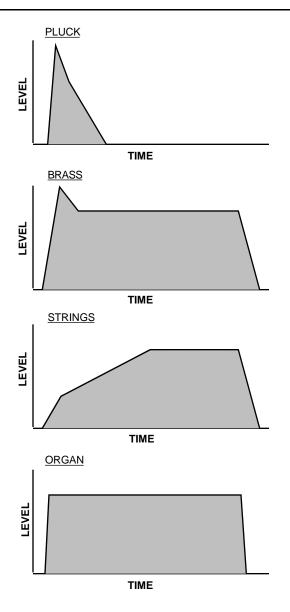
Editing any of the envelope parameters for one of the above types turns the envelope into a "USER" type.
