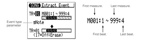
The upper "**TR**" parameter selects the source track — i.e. the track from which the event data is to be extracted: "01"  $\dots$  "16".
