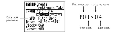
The "**TR**" parameter selects the track to be affected by the Create Continuous job: D1, D2, PC, BA, C1, C2, C3, C4.
