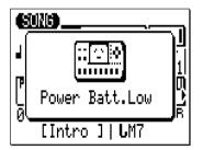
When this display appears, replace the batteries with a complete set of six new batteries. NEVER mix old and new batteries!
