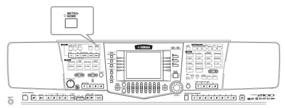
The **metronome** starts by pressing the **[METRONOME]** button. Adjust the tempo by using the **TEMPO[◄]** [▶] buttons (see below). To stop the **metronome**, press the **[METRONOME]** button again.
