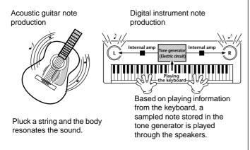
As shown in the illustration above, in an electronic instrument, the sampled note (previously recorded note) stored in the **tone generator section** (electronic circuit) is played based on information received from the keyboard, and output through the speakers.
