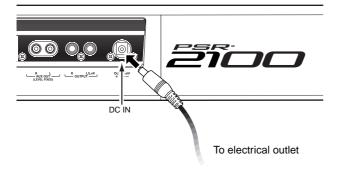
Connect the other end (normal AC plug) to the nearest electrical outlet.
