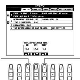
Determines the time it takes for the volume to fade in, or go from minimum to maximum (range of 0 - 20.0 seconds).
