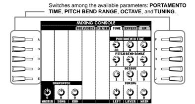
Portamento is used to create a smooth transition in pitch from one note to the
