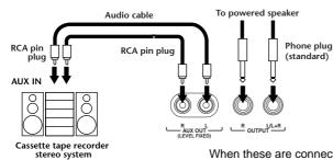
When these are connected (with RCA pin plug; LEVEL FIXED), the sound is output to the external device at a fixed level, regardless of the [MASTER VOLUME] control setting.
