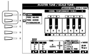
Determines the base note for each scale. When the base note is changed, the pitch of the keyboard is transposed, yet maintains the original pitch relationship between the notes.
