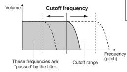
In addition to making the sound either brighter or more mellow, Filter can be used to produce electronic, synthesizer-like effects.
