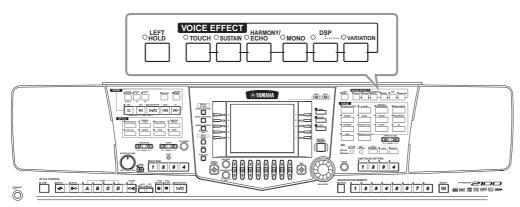
Press one of the effect buttons to turn the corresponding effects on. Press it again to turn the effect off. For explanations on each of the effects, see below.
