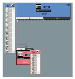
■ Connecting multiple cables simultaneously as a group
