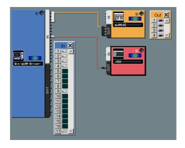
You can connect the MIDI OUT connector on the mLAN16E (an S400-compatible device) only to the computer's MIDI IN 1-16 (dedicated for an S400-compatible device). Similarly, an S200-compatible device can be connected only to the computer's MIDI IN 17 (dedicated for an S200-compatible device).
