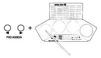
If you wish, you can simply enter the number of the instrument instead of tapping the pad repeatedly. To do so, press and hold either of the PAD ASSIGN buttons, tap the pad you've selected once, then enter the number of the desired instrument using the number buttons ⑦. (Be sure to enter two digits.)
