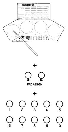
Release the PAD ASSIGN button when you hear the instrument you want. The DD-8 will now play the newly assigned instrument whenever you play the pad in question. Repeat steps 1 through 4 to assign new instruments to the other pads.
