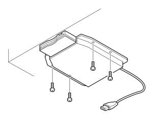
4 Connect the USB cable to the [USB TO DEVICE] terminal.
