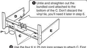
Use the four 6 × 25 mm long screws to attach C. First attach one side panel, then attach the other side panel.
