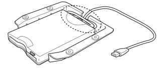
Attach the drive and case assembly to the left underside of the instrument, using the included four screws (4 mm x 10 mm).
