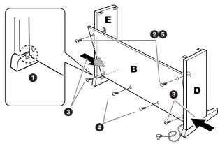
Securely tighten the screws on C that were attached in Step 2-3.
