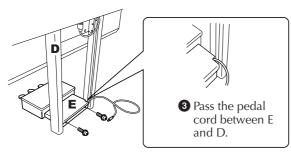
4 Make sure that E lays flat, with no gap between itself and the floor, then affix the E using two screws.
