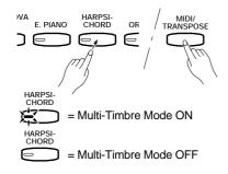
The Multi-Timbre mode is a special mode in which the Clavinova voices can be independently controlled on different MIDI channel numbers by an external MIDI device. The Multi-Timbre mode can be activated as follows:
