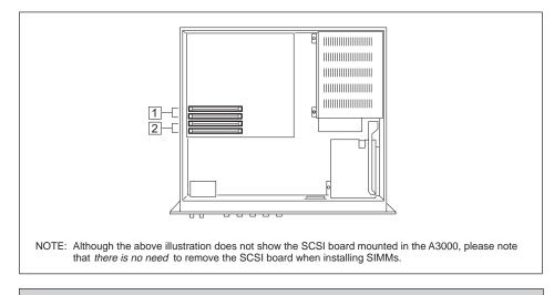
If you are using different SIMM sizes in the two banks, the larger size must be installed into the Bank 1 sockets to ensure that the A3000 handles the memory correctly. For example, if you are adding one pair of 32MB SIMMs and one pair of 8MB SIMMs, you must install the 32MB SIMMs into Bank 1. If you already have SIMMs installed in Bank 1 and are now adding a larger pair, you will need to move the original pair into Bank 2 and insert the new pair into Bank 1.
