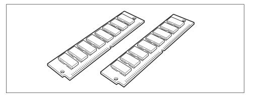
You can increase the A3000's sampling memory by installing commercially available SIMMs (single in-line memory modules). This section explains how to carry out the installation.
