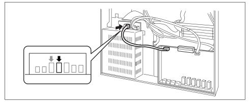
The expansion board is now fully installed. There is no need to remove the expansion board when installing other devices.
