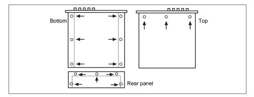
5. Hold the two sides of the cover and slide the cover straight back (over the rear panel) and off.
