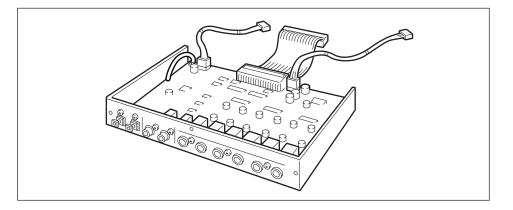
The optional AIEB1 Input/Output expansion board adds digital I/O (both optical and coaxial formats) and six assignable outputs to the A3000. For information about the board's connectors and general board setup, refer to information elsewhere in this manual (#22 to 26).
