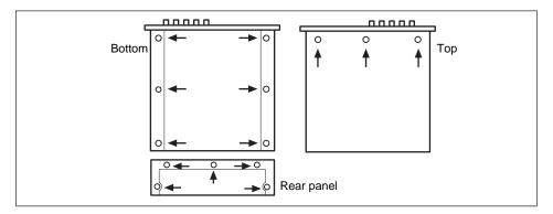
**4.** Hold the two sides of the cover and slide the cover straight back (over the rear panel) and off.
