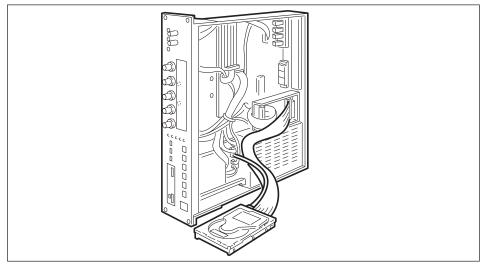
Now support the hard disk in the correct position with one hand (on the inside of the unit) while using the other hand to insert the screws and fasten into place. Note that the screws must be inserted from the outside of the unit, through the base (see drawing)
