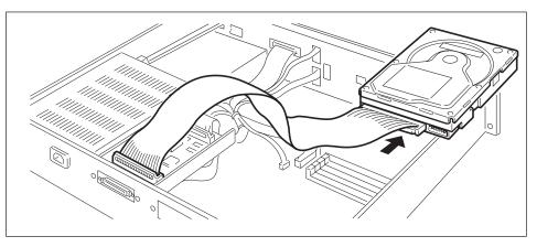
8. Using the red/white cable (hard disk power supply cable), connect the hard disk to the A3000.
