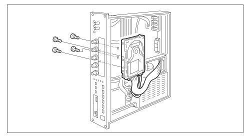
The hard disk is now fully installed. There is no need to remove the disk when installing other devices.
