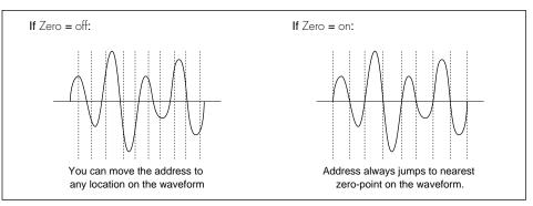
Setting an address on a non-zero point may cause the sample to "click" during playback. Forcing the address to a zero-point will ensure that you avoid this unwanted click.
