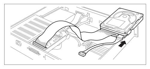
Now connect the other end of the cable into the connector indicated in the drawing. If you do not have an AEIB1 I/O expansion board installed, you can connect to either of the free connectors. Note that the connection can be made in one direction only; make sure that the direction is correct and do not try to force the connector in.
