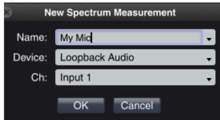
2. Select the input device and the channel that will be used to connect your measurement microphone. Give a unique name to this measurement (in this example, "My Mic").
