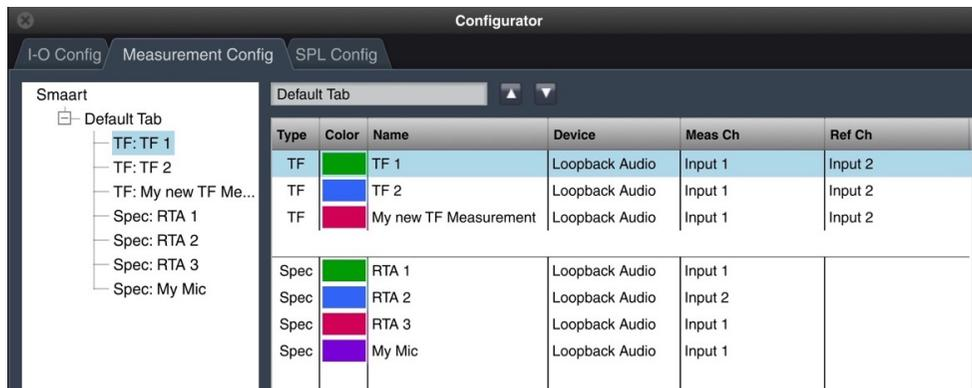
3. Click **OK**. A new spectrum measurement is created with this name. Note that the measurement, "My Mic," now appears in the Measurements list.
