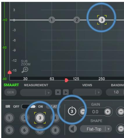
Select a band by clicking on its band number on the graph (graph markers 1–8), or by clicking the corresponding band number in the Band Selector section.
