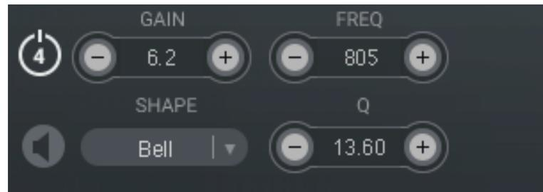
The Bell shape at narrow Q settings will become a “peak filter” for positive dB values and a “notch filter” for negative dB values.
