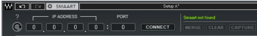
When Smart and TRACT are not connected, the displayed IP address is not valid and “Smart not Connected” is shown in the status cell.
