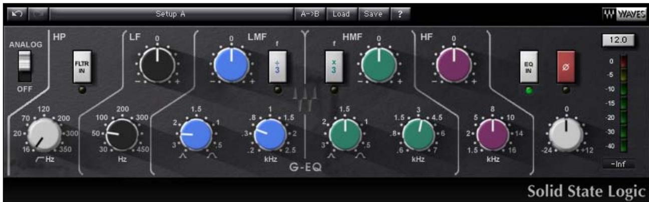
1. **High pass filter** (white knobs on the left) 18 dB/octave, 16 Hz – 350 Hz. Filter in/out switch, with indicator.
