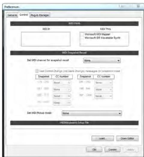
Select the desired MIDI/Keyboard Setup file. The mapping you assigned with Remote Controller Editor will become available to MultiRack.
