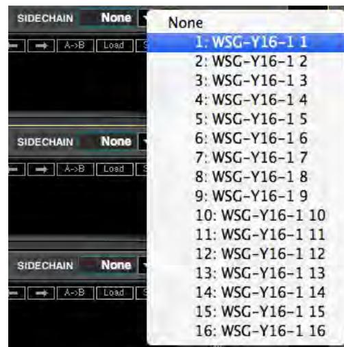
Select the input source you want to feed as sidechain to the Rack. Insert a sidechain-capable plugin. Sidechain-capable plugins are marked by a yellow **SC** button.
