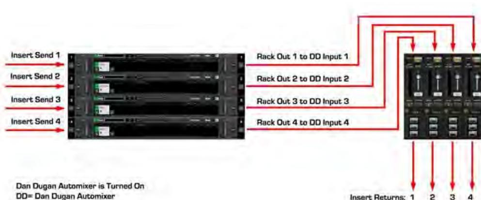
All available Outs are routed through the Dugan Automixer consecutively; Rack Outs routing values are thus identical to Automixer's channel number: Rack 1 Mono Out 1 connects to Automixer channel 1; Rack 2 Stereo Outs 3-4 connect to Automixer channels 3 and 4.
