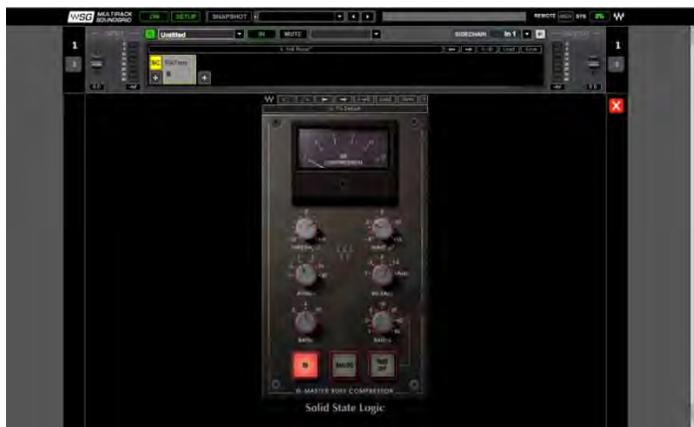
This is where you adjust each plugin. If you're already familiar with Waves plugins, this window will be very easy to use. At the top of each plugin window is a WaveSystem Toolbar, used to load, save, and compare processor settings. The layout of the WaveSystem Toolbar may vary from one plugin to another. Use this toolbar to save plugin or Rack-specific presets.
