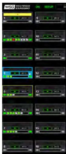
The Overview Window tells you if a rack or an individual plugin is functioning and enables you to turn on or off, bypass, or mute a Rack. Clipping is also indicated for each Rack. Use the **Overview** Window when you want to keep an eye on the entire processing setup. Since each mini-Rack in the Overview Window displays clipping information, you can easily watch out for over-level clipping across your entire setup.
