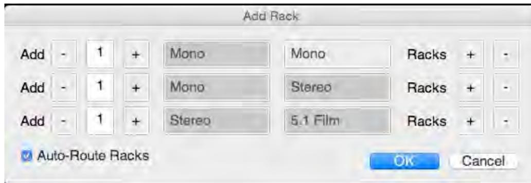
Checking the **Auto-Route Racks** option assigns input and output channels to all of the added Racks consecutively, starting from the highest currently available channel.
