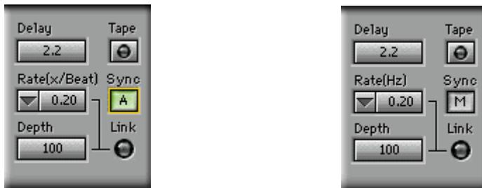
A new control labeled “Sync” has been added. Sync has two modes: A (Auto) and M (Manual).
