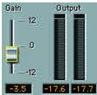
In most cases you'll leave the Gain fader on zero unless you have high-level input signals. However, some settings with higher Feedback and Inverse phase settings can produce rather large increases in peak values, so you might have to reduce the Gain even further to avoid clipping. With some settings or high-level inputs, audible clipping can occur internally even if not indicated on the output clip meters.
