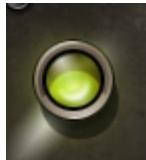
**SENSITIVITY LED** indicates when appropriate levels are reached: LED Off (too low), Green (good), Yellow (optimal), Red (very hot)
