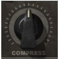
**COMPRESS** controls dynamics processing. Turning the knob clockwise results in more compression.
