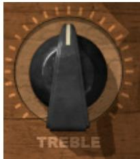
**TREBLE** controls the high frequency gain.
