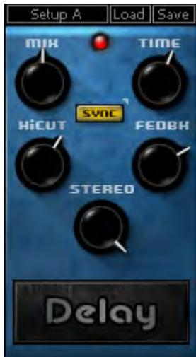
**Mix** controls the balance between Wet and Dry signal. At 50, the Wet and Dry paths mixed are mixed evenly at -3dB.
