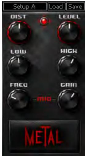
**DIST** controls the amount of distortion applied to the signal.
