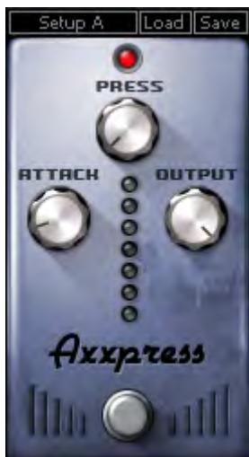
**PRESS** controls threshold and makeup gain simultaneously.
