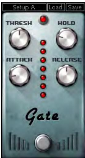
**THRESHOLD** controls the sensitivity of the gate.
