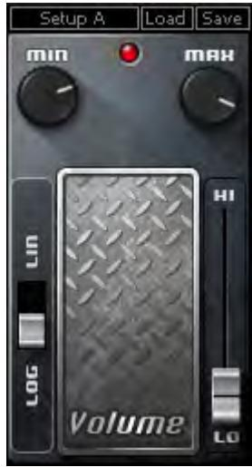
**VOLUME BAR (HI > LO)** controls output level. The position between Hi and Lo determines output volume according to the selected scaling.
