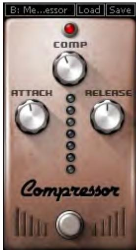
**COMP** controls the amount of compression applied to the signal.
