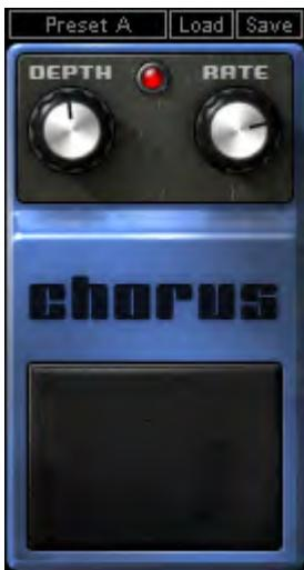
**DEPTH** controls the amount of detune effect applied to the signal.
