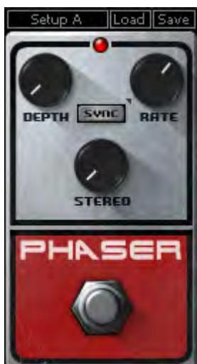
**DEPTH** controls the amount of effect applied to the signal.
