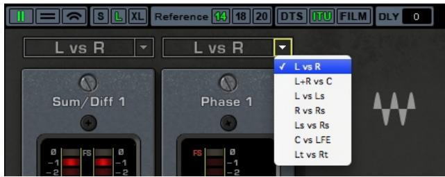
The Surround Edition plug-ins features a special single Sum & Diff / Phase page, which allows the selection of channel pairs to be displayed on two sets of Sum & Diff / Phase Meters.
