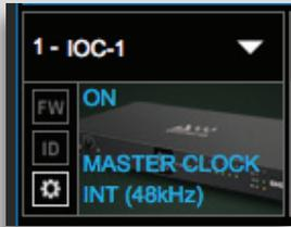
When Clock Source is set to Internal, you can use the Sample Rate menu to control the clock of the IOC device. If the IOC is the network (SoE) clock master, as determined in the Device Racks of SoundGrid Studio, then this setting determines the sample rate of the SoundGrid network.
