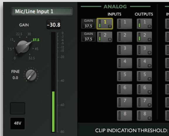
Use the Focus section to set preamp levels and turn the 48v phantom on and off.
