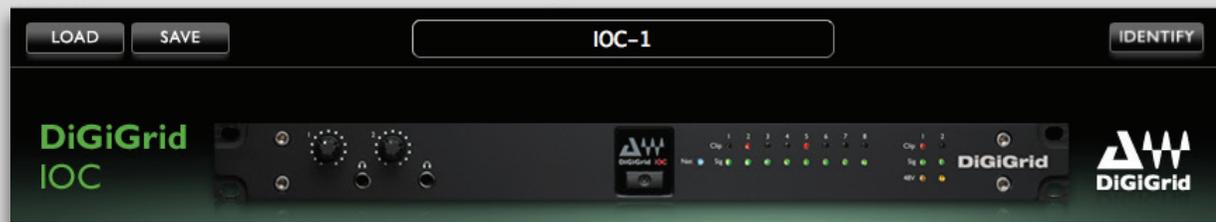
Use the Identify button to determine which IOC hardware device belongs to this Control Panel. Clicking the button causes the Network LED on the front panel of the IOC to flash in a rather psychedelic manner.
