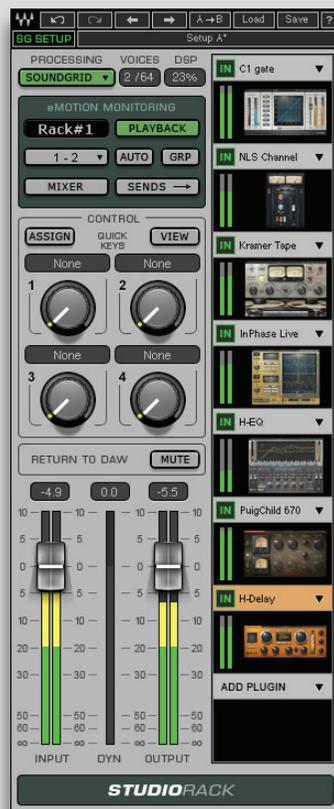
When part of a SoundGrid network with a SoundGrid DSP server, StudioRack can shift plugin processing away from the local CPU and direct it to the SoundGrid DSP server. StudioRack works in conjunction with the eMotion ST mixer to create numerous personalized monitor mixes that use the same plugins heard in the mix—all with virtually no latency.
