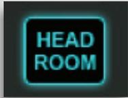
In addition to meters and clip and peak indicators—which are identical to the input controls—there is a Headroom switch that provides a -10 dB pad.
