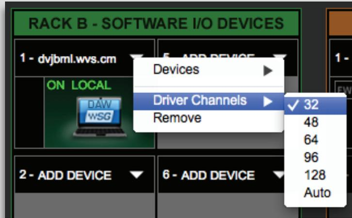
When you configure your host application, you can allocate between 32 and 128 driver channels. This is done in Rack B of the Setup page. The number of channels you select here is reflected in the Patch page: fewer allocated channels means fewer channels visible.
