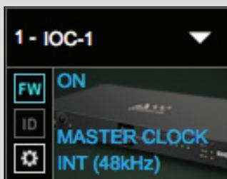
Click on the FW button to launch the firmware updater, which will initiate a scan of the hardware and then offer options. Do not disconnect the device or turn off the computer until you see “Done.” After updating, turn the IOC off and back on to reset the device.
