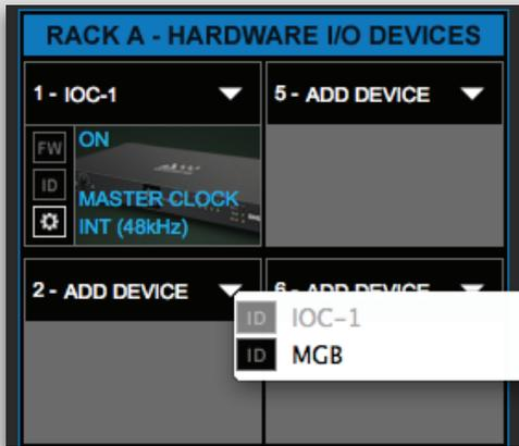
To add another SoundGrid device, click on the arrow in an empty rack slot. From the list of available devices, choose the one you want to add, in this case a DiGiGrid MGB coaxial MADI interface. In this image the IOC is grayed out, signifying that it is unavailable since it is already claimed (in this case by you).
