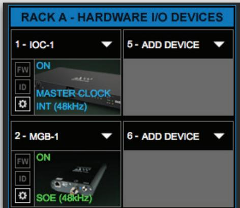
The new device is visible in the rack slot. Unless changed by the user, it remains a clock slave and is colored green. Use the same menu to change the clock master assignment from one device to another or to remove the device from the rack slot.
