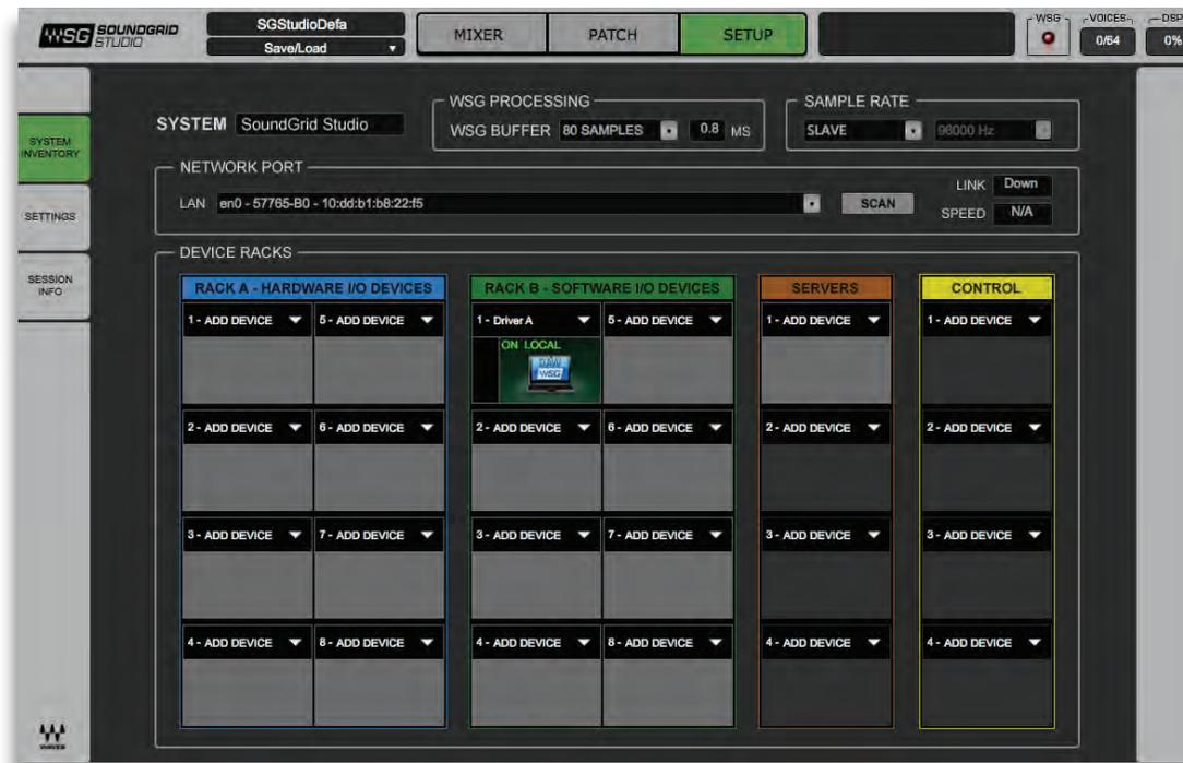
The first time you launch SoundGrid Studio, the Wizard will open. It scans the network, inventories its assets, and then configures the devices. If the Wizard does not start automatically, click the Start Auto Config button, which is next to the Network Port. Choose "NEXT" to start automatic configuration. This will take a few moments. Choose "CANCEL" to configure manually.
