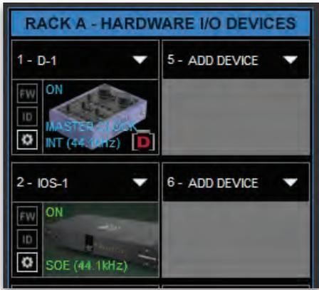
The new device is visible in the rack slot. Unless changed by the user, it remains a clock slave and is colored green. Use the same menu to change the clock master assignment from one device to another or to remove the device from the rack slot.
