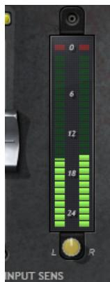
**Input Meter** displays input signal peak level.
