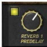
**Pre Delay 1** controls the pre-delay timing of Reverb 1. (*Settings sync to the session BPM.*)
