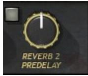
**Pre Delay 2** controls the pre-delay timing of Reverb 2. (*Settings sync to the session BPM.*)
