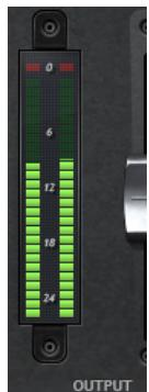
**Output Meter** displays output signal peak level.
