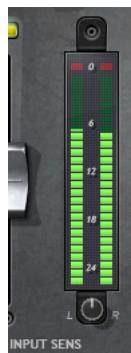
**Input Meter** displays input signal peak level.
