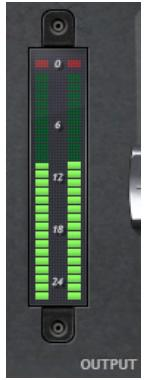
**Output Meter** displays output signal peak level.
