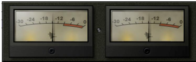
The API 550 meters display output level in dBFS. The LED located between the two meters lights up when output signal is clipping.
