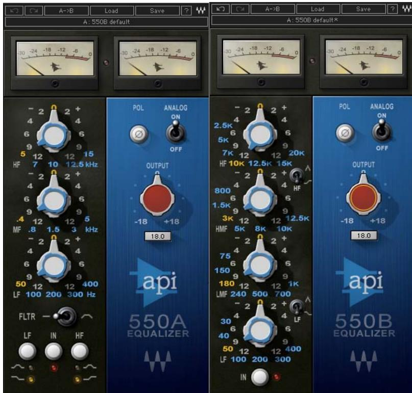
The Waves API 550 consists of the API 550A, a 3-Band parametric equalizer with 5 fixed cutoff points per band and the API 550B, a 4-Band parametric equalizer with 7 fixed cutoff points per band.
