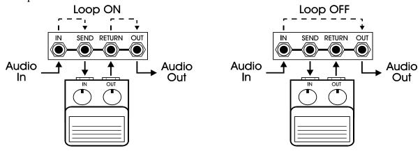
In this example, when the loop is ON, the pedal is active. When the loop is OFF, the pedal is bypassed.
