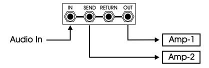
When the loop is OFF, Amp-1 plays. When the loop is ON, Amp-2 plays.
