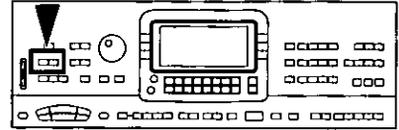
The **COMPOSER** enables you to create your own accompaniment patterns or to edit preset accompaniment patterns. A pattern is comprised of five parts: **DRUMS**, **BASS** and three **ACCOMP** parts. These parts would form the backing of a song, for example: Drums, Acoustic Bass, Piano, Jazz Guitar and Vibes. You may find it useful at first to copy and edit a preset pattern.
