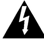
The lightning flash with arrowhead symbol, within an equilateral triangle, is intended to alert the user to the presence of uninsulated "dangerous voltage" within the product's enclosure that may be of sufficient magnitude to constitute a risk of electric shock to persons.
