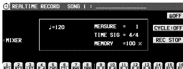
6. Use the buttons below the display to turn on the "REC" indication above the track numbers you are going to record.
