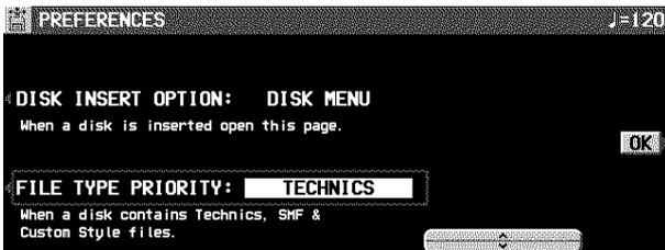
2. Use the buttons to the left of the display to select the item, and the ^ and v buttons to change the setting.
