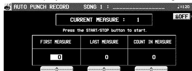
2. Use the FIRST MEASURE  $\wedge$  and  $\vee$  buttons to specify the number of the punch-in measure.
