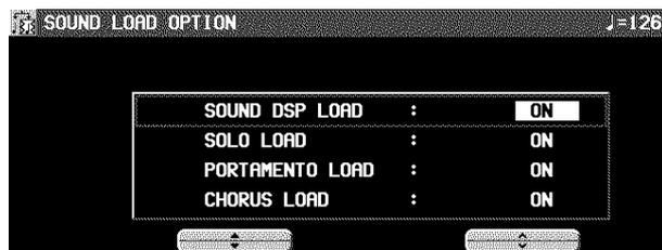
2. Use the  $\blacktriangle$  and  $\blacktriangledown$  buttons to select an item. Use the  $\wedge$  and  $\vee$  button to set the filter to ON or OFF.
