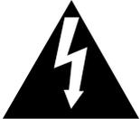
The lightning flash with arrowhead triangle symbol, within an equilateral triangle, is intended to alert the user to the presence of uninsulated "dangerous voltage" within the product's enclosure that may be of sufficient magnitude to constitute a risk of electric shock to persons.
