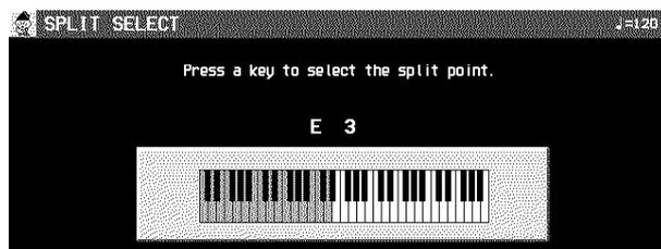
2. Press a key on the keyboard to specify the desired split point.
