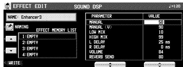
3. Use the **PARAMETER**  $\blacktriangle$  and  $\blacktriangledown$  buttons to select the parameter.
