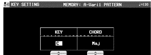
2. Use the KEY ^ and v buttons to set the key. Use the CHORD ^ and v buttons to set the chord type (Maj/Min).
