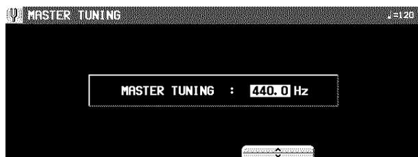
2. Use the  $\wedge$  and  $\vee$  buttons to adjust the pitch.
