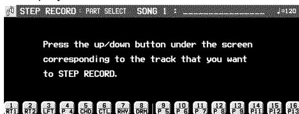
3. Use the balance buttons below the display to specify the track for the part you are going to record (only one track can be selected at a time).
