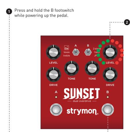
Turn the LEVEL knob on the B side to select True Bypass or Buffered Bypass.
