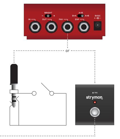
**NOTE:** Along with the knobs and toggle switches on the face of the pedal, the setting of the BRIGHT and CONFIG switches along with the bypass state of each side of Sunset is stored with the Favorite preset.
