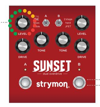
Press and hold the B footswitch until the A LED blinks.
