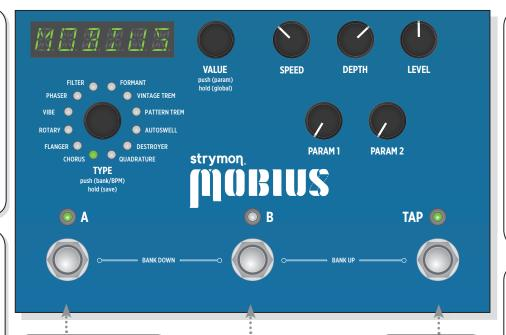
**FOOTSWITCH A:** Press to engage or bypass preset A of the current bank.
