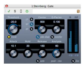
Gating, or noise gating, silences audio signals below a set threshold level. As soon as the signal level exceeds the set threshold, the gate opens to let the signal through.
