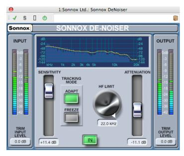
Sonnox DeNoiser is one of three plug-ins that form the Sonnox Restoration Toolkit. The tools are not just for restoring old material, but also for removing the clicks, pops, buzzes and background noise that can sometimes accidentally occur in new recordings.
