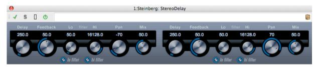
StereoDelay has two independent delay lines with freely specified delay time settings.
