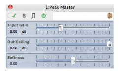
Peak master is a basic plug-in that minimizes peaks in your Audio File, allowing a louder mix without clipping. It is particularly useful in helping to tame very dynamic instruments.
