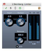
Limiter is designed to ensure that the output level never exceeds a set output level, to avoid clipping in following devices. Limiter can adjust and optimize the Release parameter automatically according to the audio material, or it can be set manually. Limiter also features separate meters for the input, output and the amount of limiting (middle meters).
