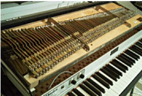
Dampers, tines and pick-ups were adjusted. Lots of tweaking and tuning lasted for almost nine months!
