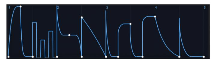
The Envelope Zoom has a special <u>CHAOS</u> feature, which can randomize the envelope's shape. CHAOS can also be set to automatically change on every cycle, creating constantly changing envelopes. The degree that CHAOS will affect the Envelope is determined with dedicated probability mini-sliders.
