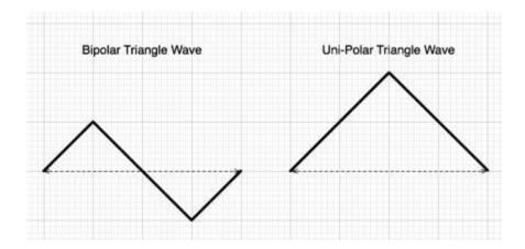
For example, a UNIPOLAR LFO applied to Oscillator pitch is great for simulating guitar-string bending, as guitarists typically bend strings only in one direction. Another use is for a UNIPOLAR LFO to modulate the Filter Cutoff. This will often create better filter sweeps than a bipolar LFO, as a bipolar LFO cycles below the mid-point—so no result is heard if the cutoff frequency is low.
