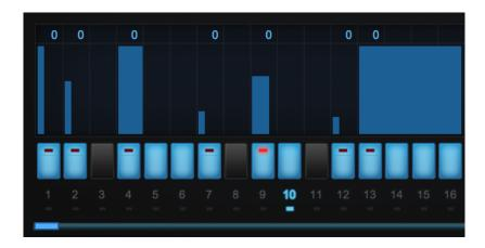
Omnisphere's ARPEGGIATOR can have up to 32 steps in a pattern. Each step can have its own length, transposition, and velocity value.
