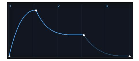
The screenshot above is from the Envelopes Zoom page, but illustrates what a standard ADSR Envelope looks like. The first to second point (or Stage) is the Attack time; the second to third point is the decay time, the third to fourth point reflects the Sustain level. After the note is released, the Sustain level drops away based on the Release time.
