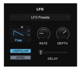
In the example below, the Oscillator's pitch is being modulated with a Triangle wave from LFO1. If LFO1 is in BIPOLAR mode, the pitch will go above, then below, the pitch of the note that was triggered. In UNIPOLAR mode, the pitch would only rise above the pitch of the note being triggered—and the range of the pitch change would be greater.
