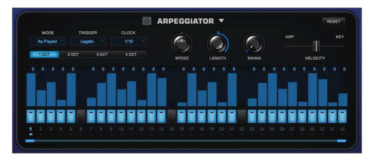
Many hardware synths include arpeggiators. An arpeggiator receives incoming MIDI notes, and outputs a sequenced pattern of notes based on a defined set of rules (such as arpeggios). Similar in concept to a step sequencer, an arpeggiator has a number of differences that set it apart. Like a step sequencer, an arpeggiator allows you to create and transpose a pattern, but it also interacts directly with the chords and intervals that you play from the keyboard.
