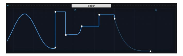
The contour of the current Envelope can be modified from this display. The point to the extreme left is always the Attack time and the last two points on the right are the Sustain level and the Release time stages. Time is represented horizontally and Level is on the vertical axis.
