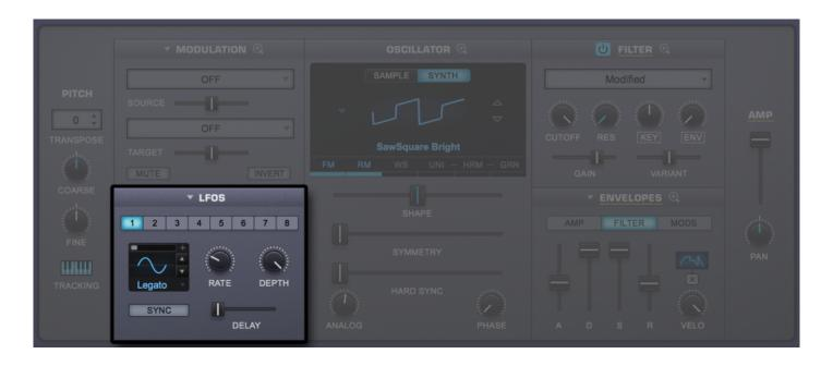
LFOs (Low Frequency Oscillators) are used for cyclical modulation effects like vibrato, tremolo, filter sweeps, and auto-pan effects.
