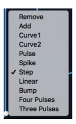
All of Omnisphere's twelve dedicated Envelopes are capable of generating contours with hundreds of points. Right/Control-clicking anywhere in the Envelope display will bring up a list that allows points to be added or removed, followed by a list of preset curves.
