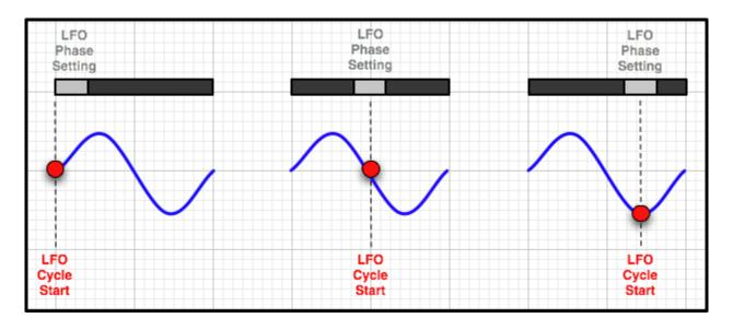
For example, if the PHASE control is in the center of the slider, the LFO will trigger from the middle of the waveform. In the screenshot above, the LFO's waveform is a sine wave, and if the PHASE control is in the center, the waveform will start at the point where the slope goes below the center-point.
