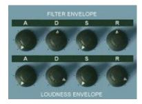
Nothing spectacular here, just an ADSR envelope for the filter on top and an ADSR envelope for the amp at the bottom. But nevertheless there is one thing to mention: The filter envelope can be used to modulate the oscillators pitch and the pulse width. The knobs for this are at the bottom left side named OM and PM (described later). This function was not present in the original.
