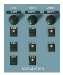
This is the section where the main LFO is controlled and routed to the desired modulation aims. For the modulation lever, there's a separate and independent sine LFO (rate control above leavers). If wished, the modulation lever can be switched back to the main LFO as it is in the original device (ADDITIONAL FUNCTIONS SECTION, "Wheel LFO").
