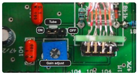
The small selector Pad to bybass the tube and the gain adjustment
