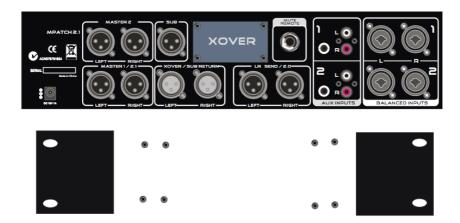
\* Note: The M-Patch 2.1 accepts mic or line level input signals. Do notconnect your power amplifier outputs to the M-Patch 2 inputs!
