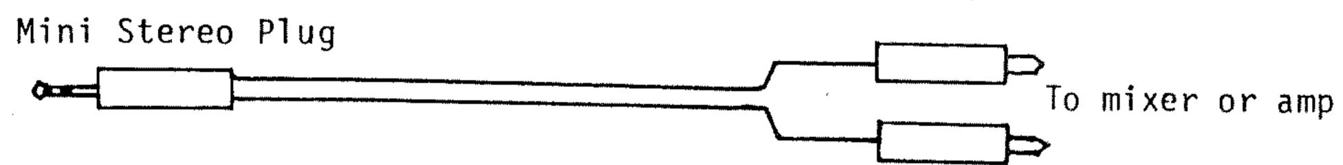
2. Use the AUX STEREO IN jack as an <u>OUTPUT</u> jack, inserting a regular unitar plug into the jack halfway, so that both channels are contacted and mixed together. Alternatively, a stereo plug with both tip and ring wired together can be inserted fully into the AUX jack. The AUX STEREO jack will drive a standard guitar amplifier, by providing a high impedance. low level output.
