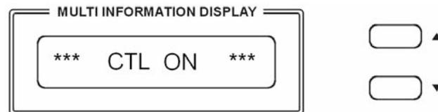
CTL ON              This configuration will allow the instrument to send and receive the Control Change Midi information.
