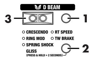
Press D BEAM [ON] button to make the button light.
