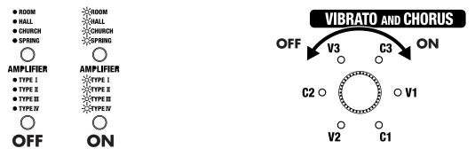
This will be ON when the [VIBRATO AND CHORUS] knob is turned to the right, and OFF when turned to the left. When you press the VIBRATO AND CHORUS [ON] button, this will return to the default setting.
