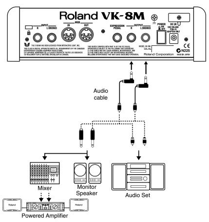
Use audio cables to connect audio equipment, such as an amp or speakers. If you are using headphones, plug them into the PHONES jack.
