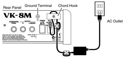
\* To prevent the inadvertent disruption of power to your unit (should the plug be pulled out accidentally), and to avoid applying undue stress to the AC adaptor jack, anchor the power cord using the cord hook, as shown in the illustration.
