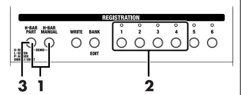
Press the [H-BAR PART] button and the [H-BAR MANUAL] button at the same time.
