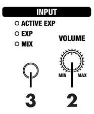
Lower the keyboard volume by turning the knob towards MIN. Raise the keyboard volume by turning the knob towards MAX.
