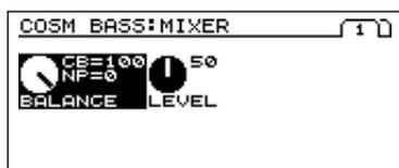
5. Turn the VALUE dial to adjust the balance between the COSM bass sound and the sound of the normal pickup.
