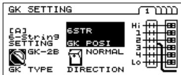
5. Turn the VALUE dial to specify the location at which the divided pickup is attached.
