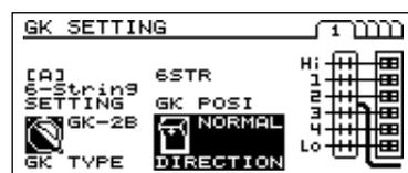
**NORMAL:** Positioned with the cable extending toward the bridge.
