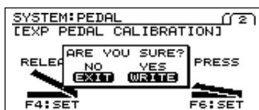
\* When you see “More Release!” on the display, please check again if the built-in EXP pedal is released to the minimum position.
