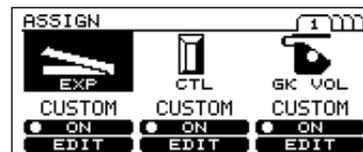
2. Press [F2] (ON/OFF) to switch the CTL pedal function on/off.
