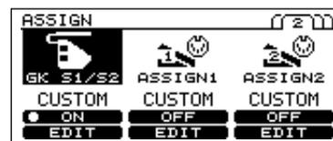
3. Press [F1] (ON/OFF) to switch the GK SW function on/off.
