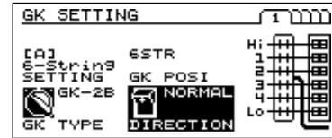
9. Turn the VALUE dial to specify the direction in which the divided pickup is attached.
