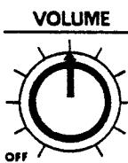
Controls volume, and is also used as power switch. Turning clockwise from OFF, power is supplied, and turning further to the right increases volume.
