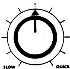
Controls rhythm tempo in a wide range from slow ( $\text{♩} = 50$ ) to quick ( $\text{♩} = 200$ ); turning clockwise increases tempo.
