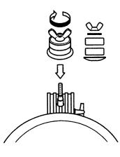
To change the MDY-7U's angle, loosen the clamp.
