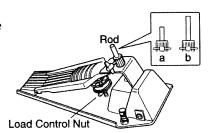
The KD-7 needs to be inserted onto the end of your kick-pedal. The beater (an accessory) should be connected as shown.
