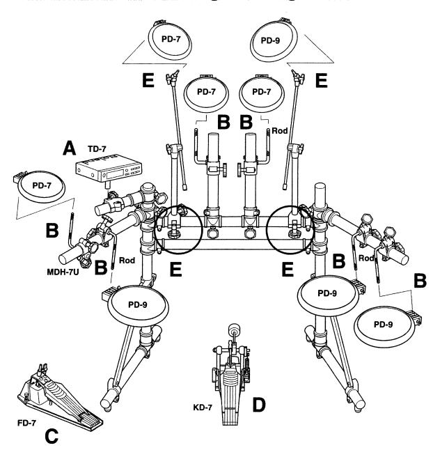
Fix the TD-7 in place using the supplied screws (M5 x 8 mm). Never use any other screws, as damage could result to the TD-7.
