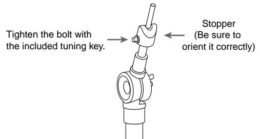
2. Attach the CY-6 so the unit is oriented as shown in the diagram.
