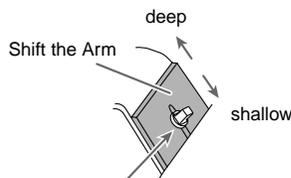
Loosen the nut with the included tuning key. After adjusting, tighten the nut.
