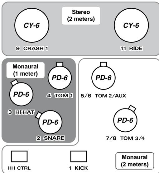
Using the provided cables, connect the pads, cymbal pads, hi-hat control pedal, and kick trigger unit. Carefully refer to the numbers shown in the illustration and connect to the appropriate TRIGGER INPUT jacks on the TD-6's rear panel.
