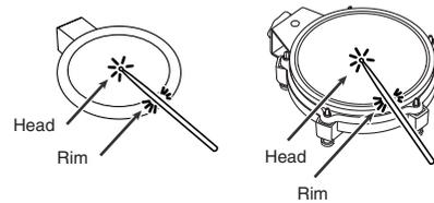
**MEMO** When using rim shots on the PD-80R, PD-105, PD-120, or PD-125, connect the pad to the SNARE trigger input jack with a STEREO cable.
