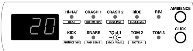
**TIP** Hold down [EDIT] and press [-] to have the indicators light in the reverse order of that when only [EDIT] is pressed.
