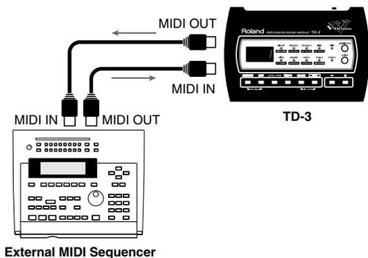
2. Hold down [INST] and turn the TD-3's power on. Local Control is set to "OFF."
