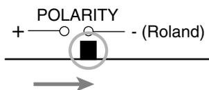
If you are using a PD-7, PD-9, or KD-7, the pad's polarity switch should be in the "- (Roland)" position. For more detailed information, refer to your PD-7, PD-9, or KD-7 owner's manual.
