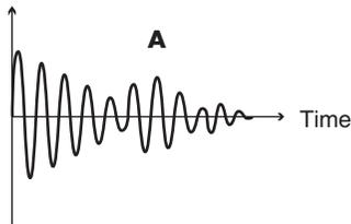
This occurs in particular at the decaying edge of the waveform. Retrigger Cancel detects such distortion in and prevents retriggering from occurring.
