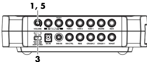
1. Turn the VOLUME knob on the TD-3's rear panel completely to the left to lower the volume to "0."
