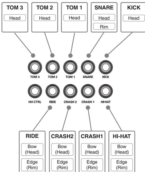
The following trigger inputs allow you to play either rim shots and cross stick on the snare pad, or cymbal edge shots and choking, and other techniques.
