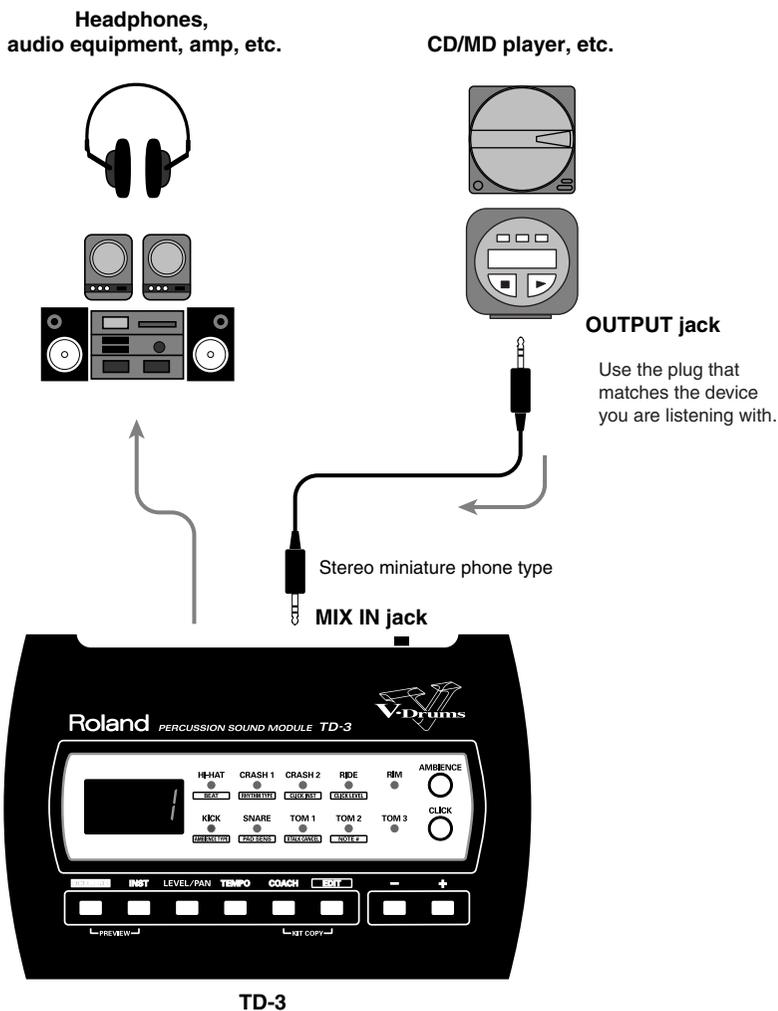
**NOTE** To prevent malfunction and/or damage to speakers or other devices, always turn down the volume, and turn off the power on all devices before making any connections.
