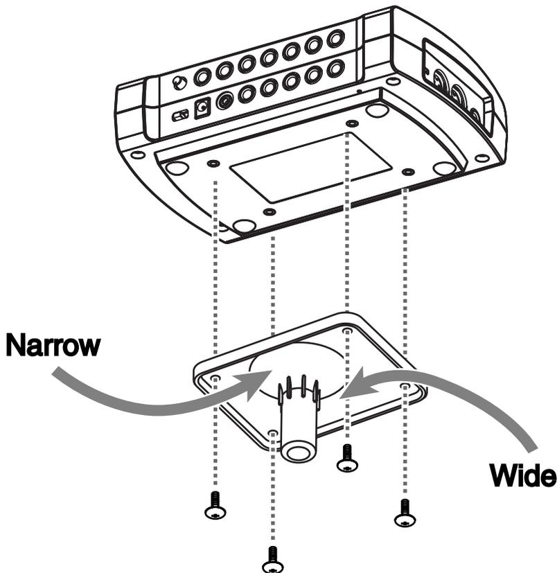
**NOTE** When turning the unit upside-down, get a bunch of newspapers or magazines, and place them under the four corners or at both ends to prevent damage to the buttons and controls. Also, you should try to orient the unit so no buttons or controls get damaged.
