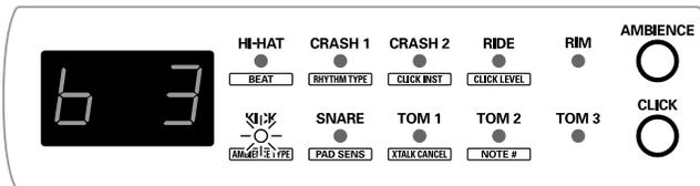
**TIP** Hold down [EDIT] and press [-] to have the indicators light in the reverse order of that when only [EDIT] is pressed.
