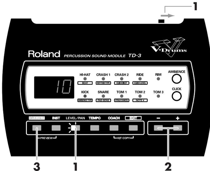
1. Be sure the POWER is OFF, then hold down [LEVEL/PAN] and turn on the power. "Pedal Modify" appears in the scroll display, then the Foot Closed level is indicated, and [LEVEL/PAN] flashes.
