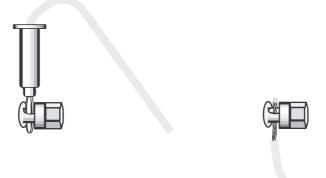
ullet Contacts for the INPUT connectors are wired in parallel. This makes it convenient when a parallel connection is desired. (Parallel Connection  $\rightarrow$  p. 9)
