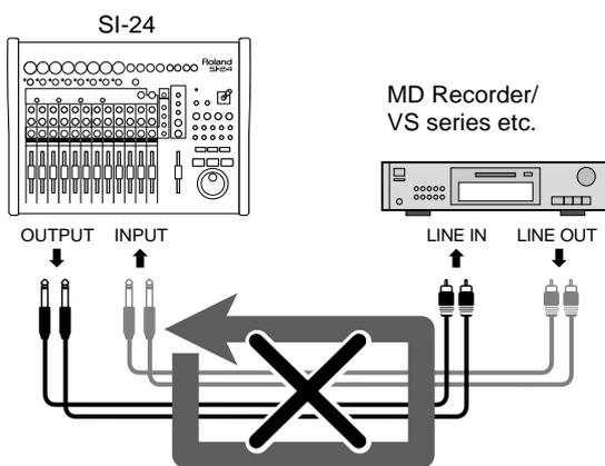
Example of a Digital Loop Connection
