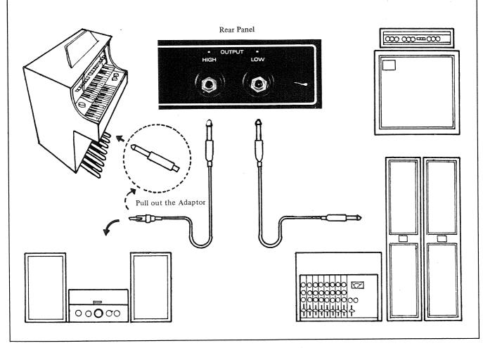
FOR PERFORMING: \* Connect the RS-101 to an amplifier and turn the power switch to ON. Set tablets for Brass and Strings I and II at the F clef (?) and G clef (§), then slide up the "Volume" control to perform.
