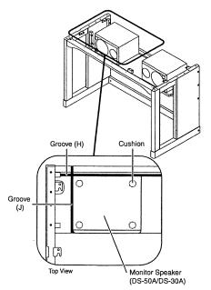
\* When installing the monitor speakers, be sure to position them so they are aligned with the grooves in the rack board.
