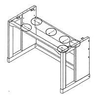
(3) Set the rack board so that the dowels (F) fit into the grooves at the front of the rack board (A).
