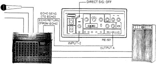
If the mixer ECHO SEND and ECHO RETURN use balanced XLR type connectors at +4dBm signal levels or levels near 0dBm, use the RE-501 balanced input and output.
