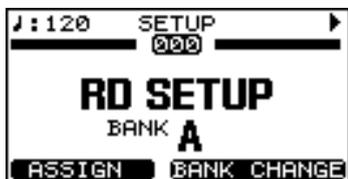
This SETUP<000> is the Setup containing the stored settings for ONE TOUCH [PIANO] or [E.PIANO]; the contents cannot be overwritten by pressing the [WRITE] as with other Setups.
