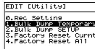
5. Press CURSOR [▲]/[▼] to select "1. Bulk Dump Temporary" or "2. Bulk Dump SETUP."
