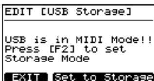
If you want to switch to USB Storage mode, press [F2 (Set to Storage)] (the instrument switches to USB mode, and the USB Storage screen opens).
