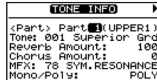
2. Press CURSOR [◀]/[▶] to switch screens, and press CURSOR [▲]/[▼] to move the cursor to the parameter to be set.
