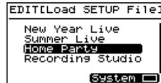
4. When loading System parameter settings, press [F2 (System)] to check in the check box.
