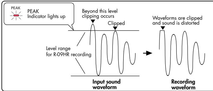
Use the [Input Level Button] to adjust the volume so that the [PEAK Indicator] does not light up even when the loudest sound is produced by the target. Doing this prevents clipping during the loudest parts of a song or during instrumental passages played fortissimo.
