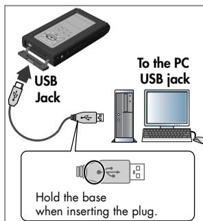
After a while, the R-09HR is recognized by the PC, and the <USB Screen> is shown in the R-09HR's display.
