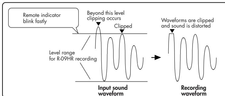
Use the [Input Level Buttons] to adjust the volume so that the remote indicator does not blink faster (clipping stage is not reached) even when the loudest sound is produced by the recording target. Doing this prevents clipping during the loudest parts of a song or during instrumental passages played fortissimo.
