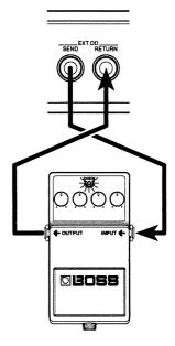
When using an external effect, select "EXTERNAL" for "TYPE." Adjust the intensity of the external effect's distortion using the controls on the external effect. Be sure the effect to be provided by the external effect is switched ON. The output levels on the external effect should be adjusted so the levels it outputs will be equal, whether the effect is switched on or off.
