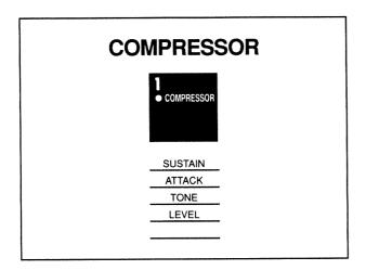
This effect compresses the higher level signals, and boosts the weaker input to equalize the volume of the sound, allowing you to obtain sustained sounds that are free of distortion.
