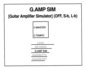
Simulates the response of a guitar amplifier. Using this, you can connect the guitar directly to a mixer (line input) and still obtain a robust sound, with no discernible loss.
