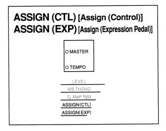
These assign, to the Control pedal and Expression pedal (optional), the functions to be used with the Control Effect function. For more information, see "Adding Effects — Control Effects" on page 12.
