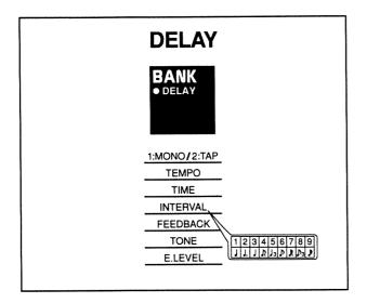
This is a versatile delay that allows you to set a delay time of up to 2.0 seconds (in monaural). It can also be used as a Tap Delay that can output signals in stereo. By using the Tempo function, you can set the delay time in real-time with a footswitch (FS-5U: optional) or the Control pedal.
