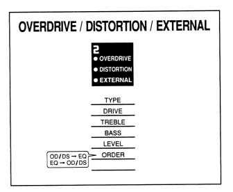
These effects are used for distorting sounds and creating a long sustain. The ME-8 allows you to use the built-in Overdrive and Distortion, and to connect an external effect.
