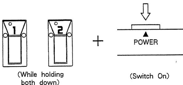
After this operation, "FP" is shown in the Display for about 2 seconds.
