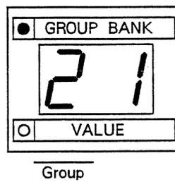
You can also select a Group by using the optional pedal switch BOSS FS-5U or Roland DP-2. Connect a pedal switch to the Group Shift Jack on the ME-5, and pressing the pedal will change the Group numbers as 1 → 2 → 3 → 4 → 1 → .....
