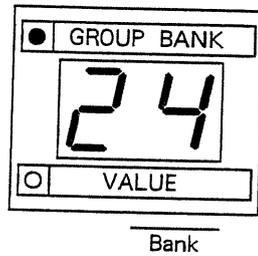
\*To cancel Bank selection mode, push the Bank Pedal while the number at the right side of the Display is flashing.
