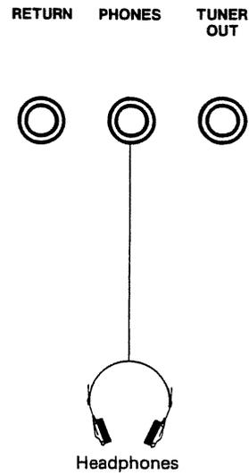
The volume of the headphones is determined by the Master Level (see page 41). If the output level from the headphones is too high or low, edit the value of the Master Level parameter.
