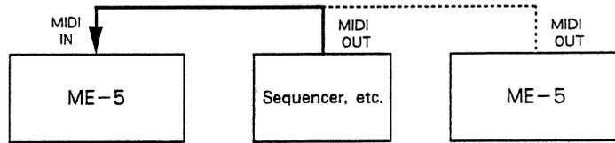
Now, the Patches on the ME-5 are automatically changed by receiving data (Exclusive Message) from the transmit device. ("Current Bulk Load" changes only one Patch.)
