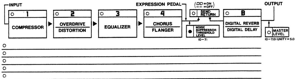
The ME-5 features high speed VCA and envelope detection circuits that activate an expander when the instrument level becomes lower than the threshold level. Therefore, extremely natural noise reduction effects can be obtained without deterioration of the sound quality or expression.
