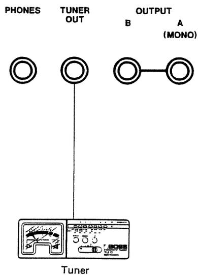
\*The Tuner Out Jack is strictly for connecting a tuning unit; do not connect any other device such as an amplifier.
