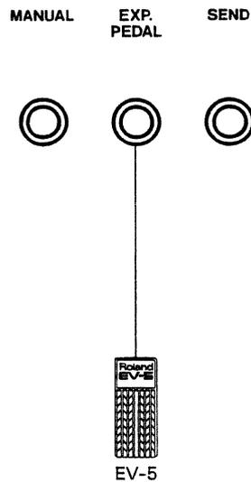
When you fully depress the Expression Pedal, the output level is equal to the normal level (output level when the Expression Pedal is not connected), while it is equal to the minimum volume set on the Expression Pedal when the pedal is lifted to the highest position.
