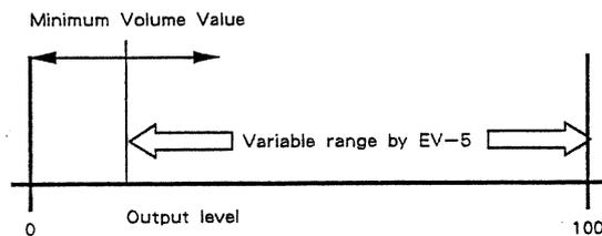
\* "100" is the output level when the Expression Pedal is not connected.
