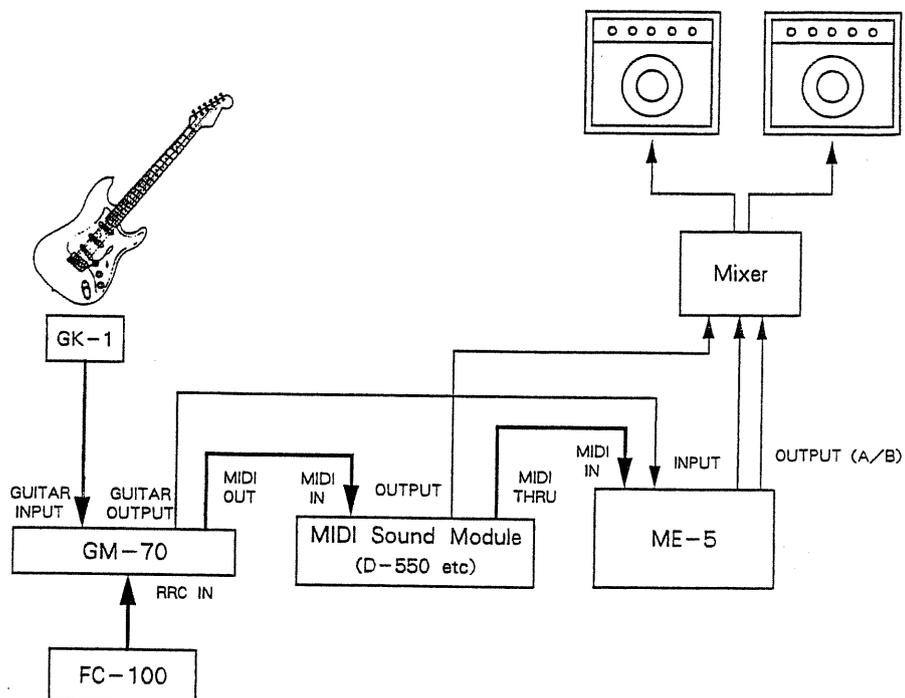
On the contrary, when the Patches on the ME-5 are changed, the corresponding Program Change number (Tx) is sent from the MIDI OUT. This means that if the external effect connected between the Send and Return Jacks features a MIDI IN connector, the effect program (=memory number) of that effect will be simultaneously changed also.
