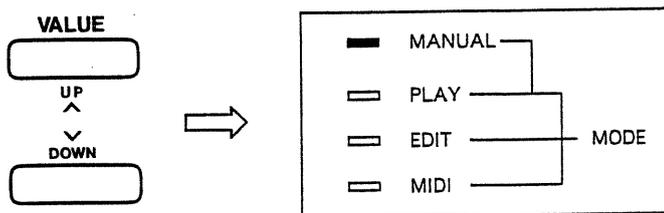
(Press both buttons simultaneously)
